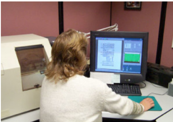
Fig. 2. Kelly Lauren monitors input from the Mekel scanner after feeding fiche through the clear plastic portal on the left. The green square on the right represents the entire microfiche, and the larger image shown on the left is one page scanned from it.
