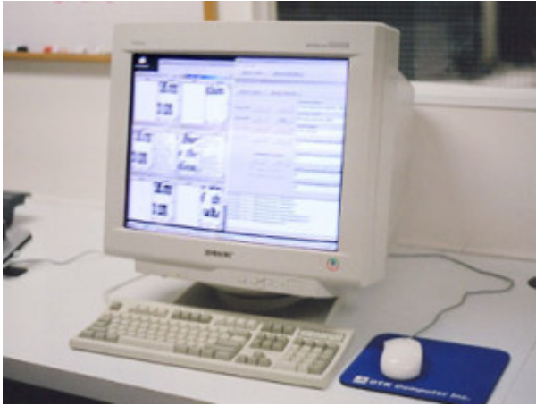
Fig. 4. Standing solo in another room, the computer running the OCR software “reads” and translates text at a rate of ten seconds per page. The rectangles with large black characters show close-ups of pages while the rectangles with smaller gray characters next to them display the ASCII text as it is generated.
