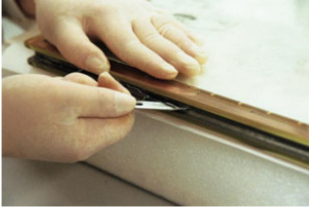
Fig. 2. Gloved hands slowly work the blade back and forth, through the lead seal that holds the top and bottom sheets of encasement glass together. Photograph by Earl McDonald, courtesy of the National Archives and Records Administration.
