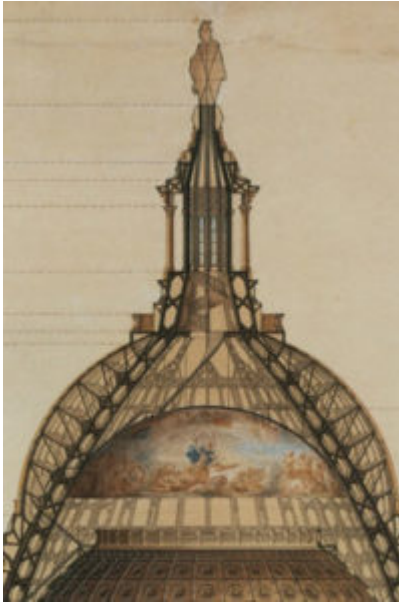
Fig. 15. Detail of “Cross-Section of the Dome of the U.S. Capitol,” Thomas U. Walter (1859). Courtesy of the Architect of the Capitol, Washington, D.C. Click image to enlarge in a new window.
