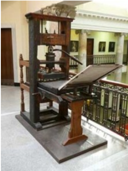
Fig. 1. The Isaiah Thomas printing press, built in London in 1747, restored to its present condition in 1977, and now resident at the American Antiquarian Society, Worcester, Massachusetts. Photograph courtesy of the author.
