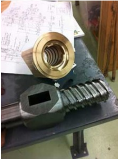
Fig. 7. The spindle and nut cut by my college machinist for the replica press. Note the three-start thread visible on the nut and the plans from Harris and Sisson's The Common Press in the background. Photograph courtesy of the author.
