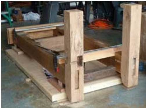
Fig. 8. The cheeks of the replica press locked up in jigs to keep the inner faces of the cheeks parallel to one another as I fitted pieces such as the head, till, and foot assembly. Photograph courtesy of the author.
