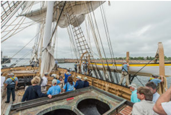
2. The tryworks on the C.W. Morgan. Photograph © Mystic Seaport, Mystic, Connecticut.
