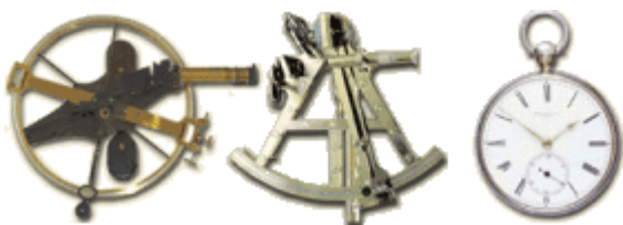
Fig. 3. Examples of the kinds of instruments used by Frémont, from left to right: a reflecting circle, a sextant, and a chronometer. Courtesy Bob Graham, www.longcamp.com .
