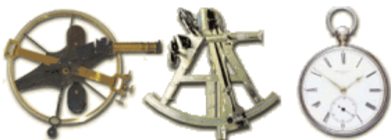
Fig. 3. Examples of the kinds of instruments used by Frémont, from left to right: a reflecting circle, a sextant, and a chronometer. Courtesy Bob Graham, www.longcamp.com .
