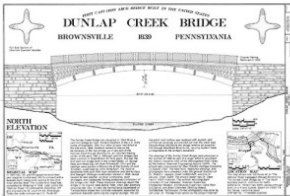
Fig. 1. Applying principles advocated by Paine, the designers of the first iron arch bridge in the United States created a structure that is still in service. Historic American Engineering Record, National Park Service, delineated by Christopher H. Marston, 1992. Library of Congress.
